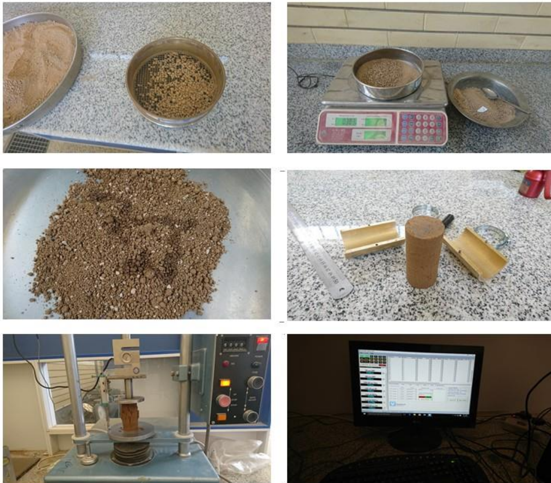
Fig. 11. Unconfined compressive strength test
