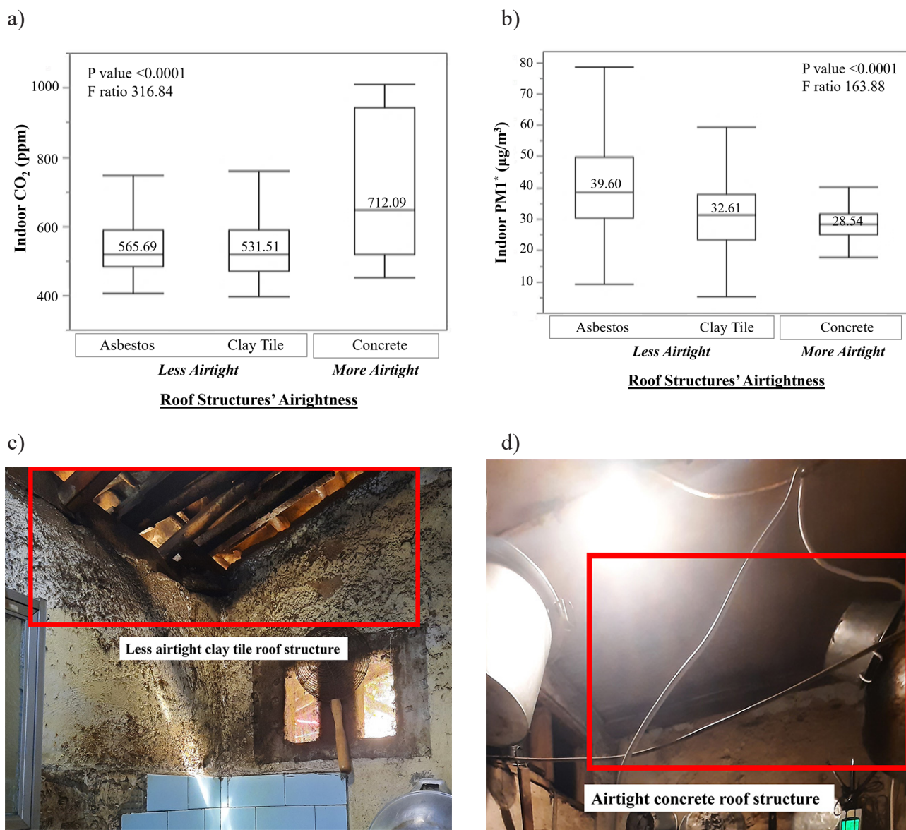
Fig. 12. Effect of roof structures' airtightness of different covering materials on (a) ANOVA for indoor CO 2 and (b) ANOVA for indoor PM 10 level, and illustration of house structure with (c) clay tile and (d) concrete covering material
