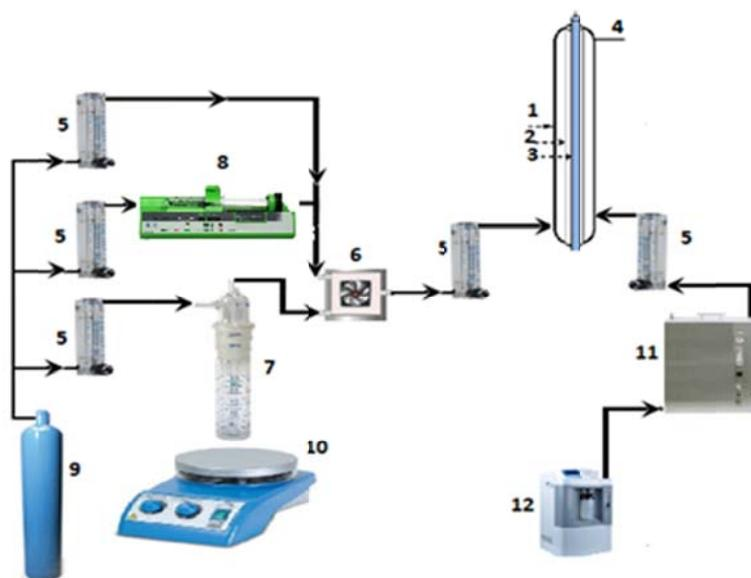
Fig.1. Schematic of setup for VUV experiments
