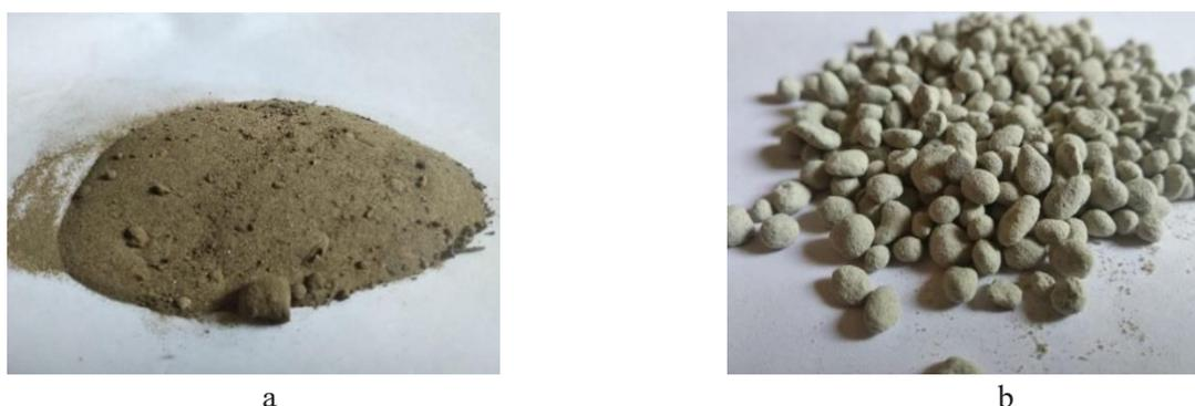
Fig. 1. a) Fly ash as Powder form; b) Fly ash as Pellets form
