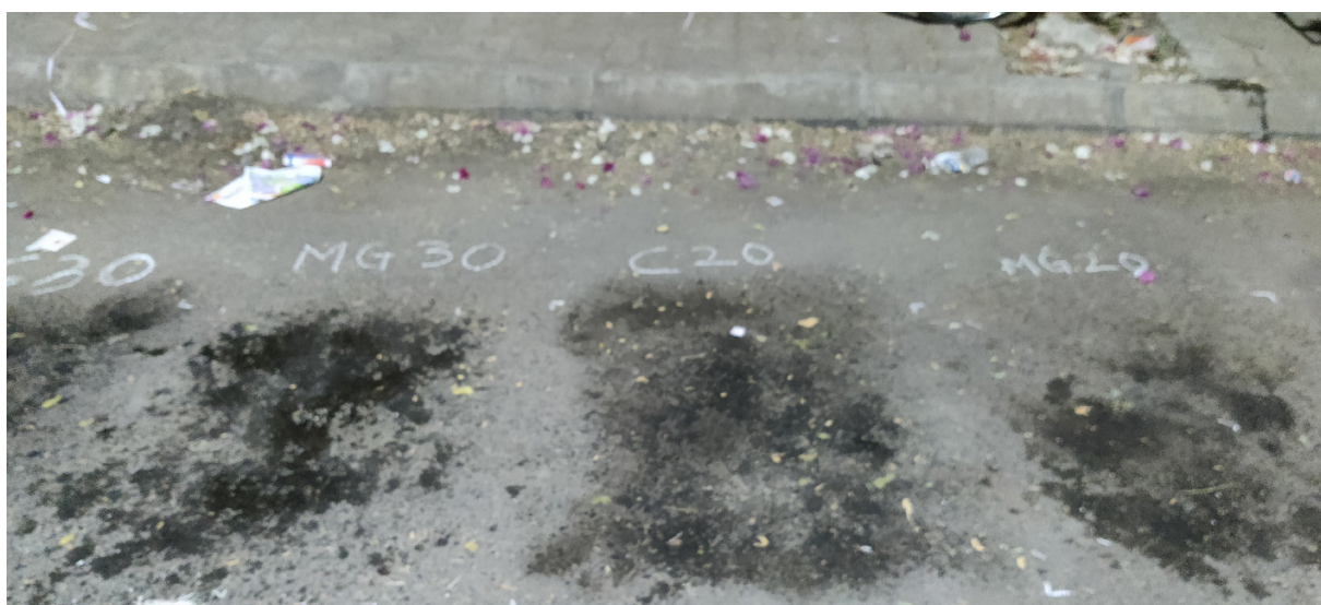
Fig. 2. \text{CaCl}_2 and \text{MgCl}_2 solutions sprayed on 1m 2 area of the road
