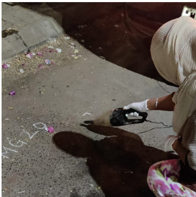
Fig. 1. Sampling being carried out along the road side with the help of portable vacuum cleaner
