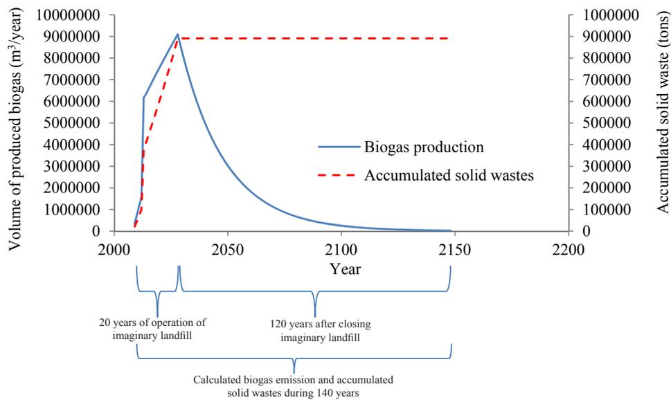
Fig. 1. Estimation of accumulated solid waste and produced biogas in the imaginary solid waste landfill of Najafabad over 140 years (2008–2148)
