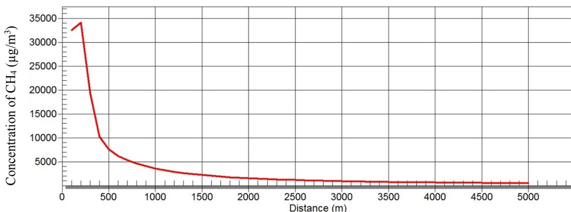
Fig. 5. Concentration of CH<sub>4</sub> in air versus distance in 2015
