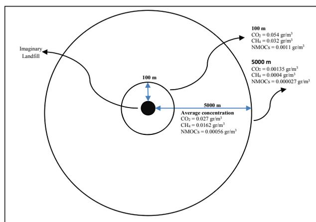
Fig. 7. Concentration of CO<sub>2</sub>, CH<sub>4</sub> and NMOCs in air at distance of 100 and 5000 m in 2015
