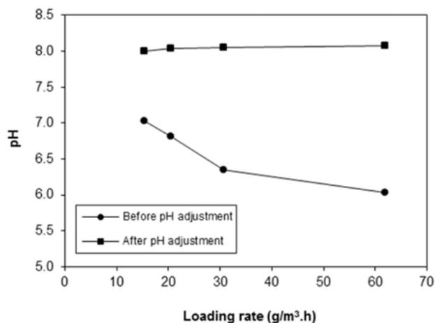
Fig. 4. Effect of loading rate on the mean daily changes in mixed liquor pH.
