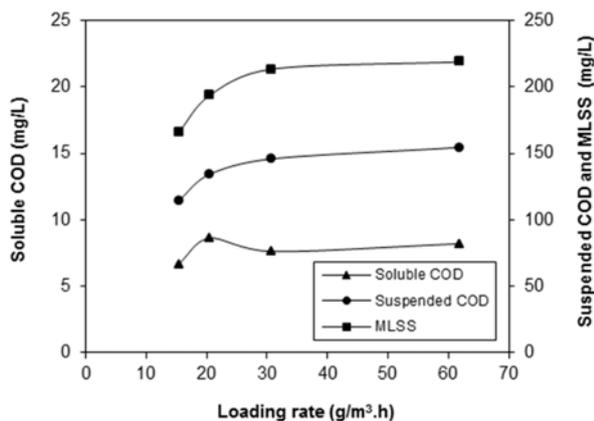
Fig. 5. Variations of the mixed liquor quality parameters (soluble and suspended COD and MLSS concentrations) at different DCM loading rate
