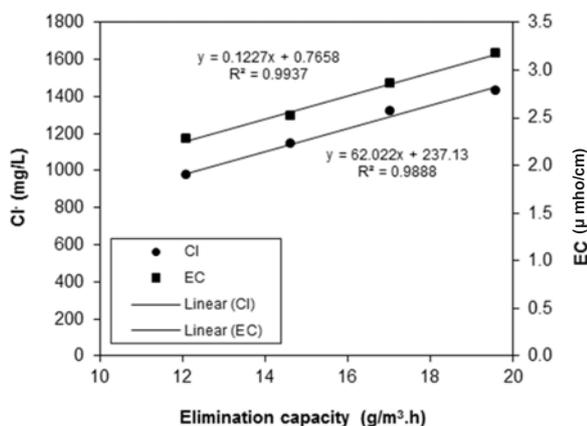
Fig. 6. Chloride concentration and EC of the mixed liquor as a function of DCM removal rate.
