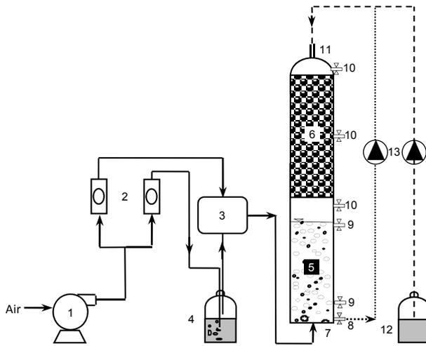
Fig. 1. The experimental set-up used in this study: (1) air compressor, (2) air flowmeter, (3) mixing chamber, (4) DCM vaporization chamber, (5) bubble column bioreactor, (6) biofilter, (7) gas inlet, (8) drainage port, (9) liquor sampling port, (10) gas sampling port, (11) gas outlet, (12) nutrient reservoir and (13) peristaltic pumps.
