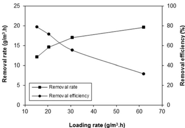
Fig. 3. Effect of DCM loading rate on the removal rate and efficiency in HBCB bioreactor.
