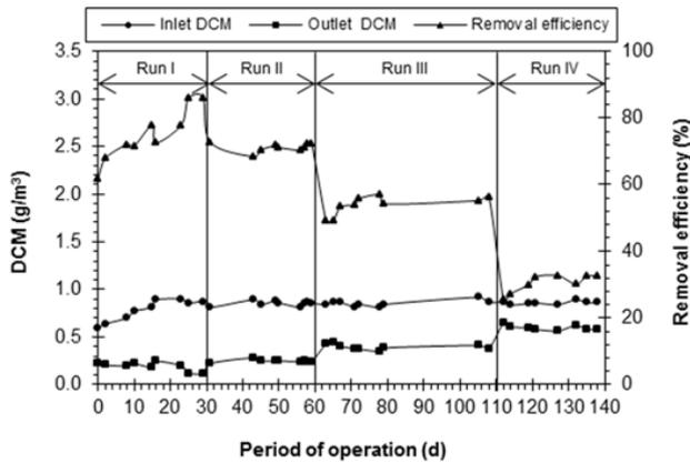
Fig. 2. The overall performance and efficiency of HBCB bioreactor in DCM removal from the gas phase.
