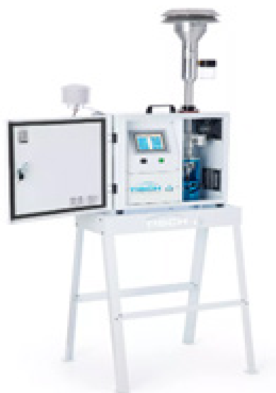
Fig. 1. Low-volume air sampler with quartz microfiber filter assembly used for indoor particle collection
