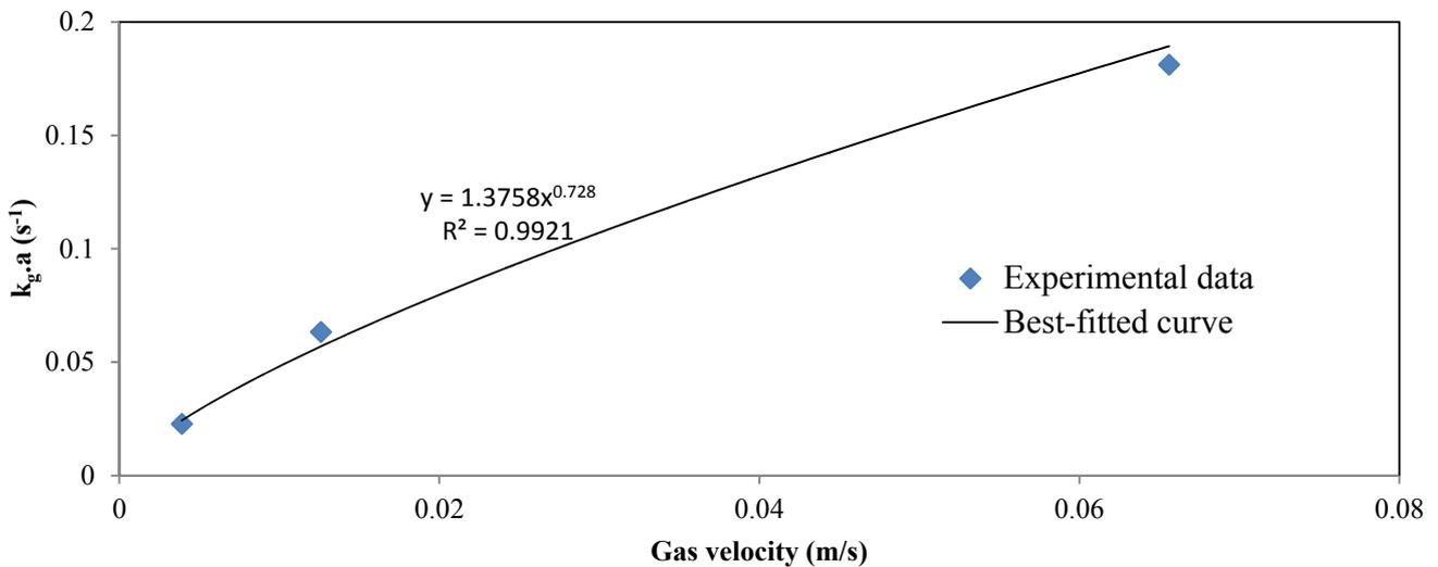
Fig.5. The variation of  $k_g \cdot a$  with gas velocity
