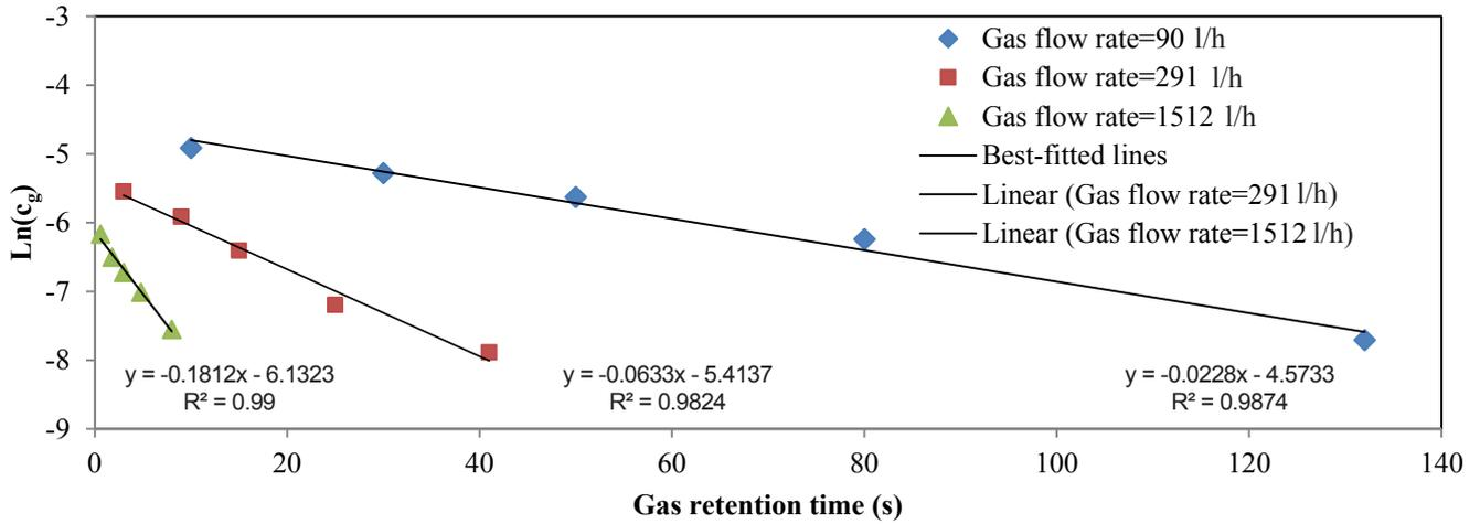
Fig.4. The plot of  $\ln(C_g)$  versus gas retention time
