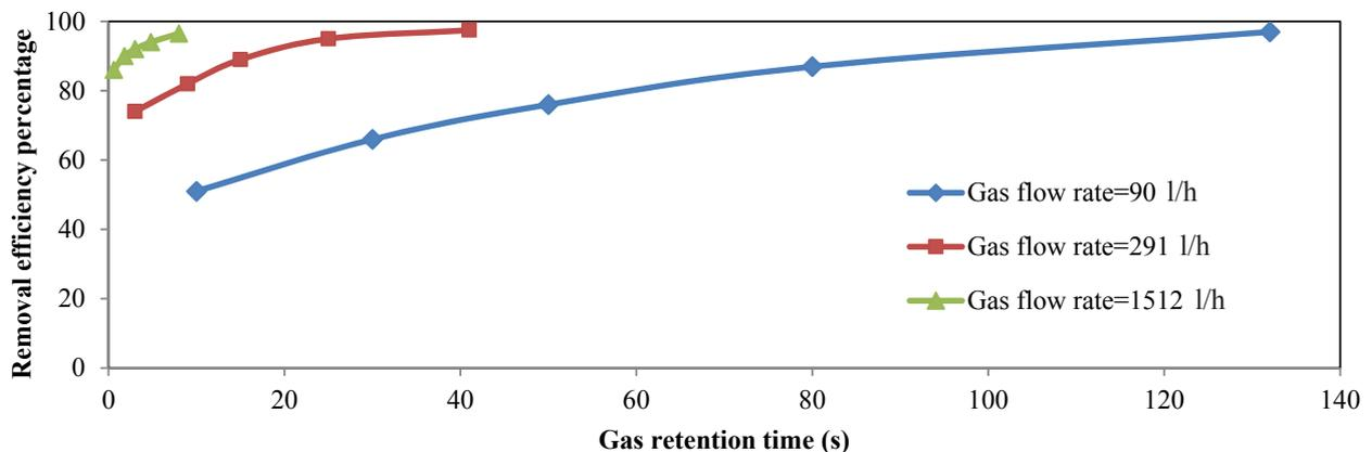
Fig.3. Formaldehyde removal efficiency versus gas retention time in the continuous BTFR for gas flow rates of 90, 291 and 1512 l/h
