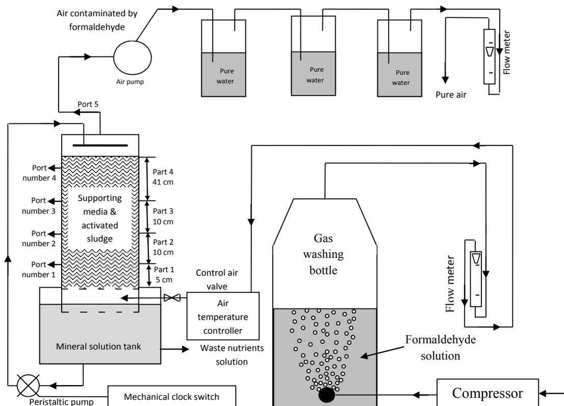
Fig.1. Schematic of the continuous BTFR and synthetic contaminated air stream (SCAS) production systems
